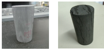
图2 岩心渗吸前后外观对比 Fig. 2 Core appearance before and after imbibition
